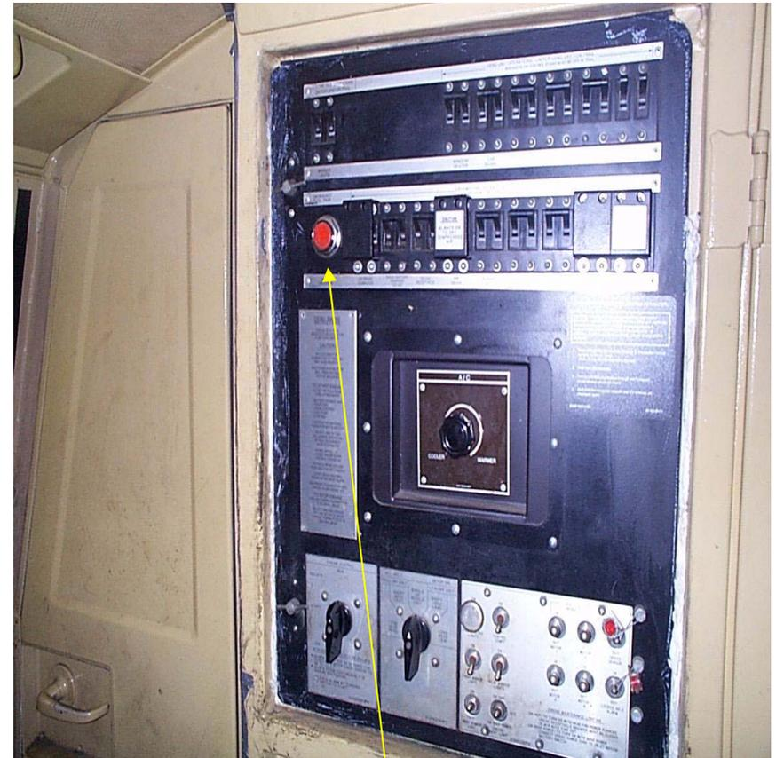
Emergency fuel Trip (shut off) on the panel on the rear wall of the engineers compartment
