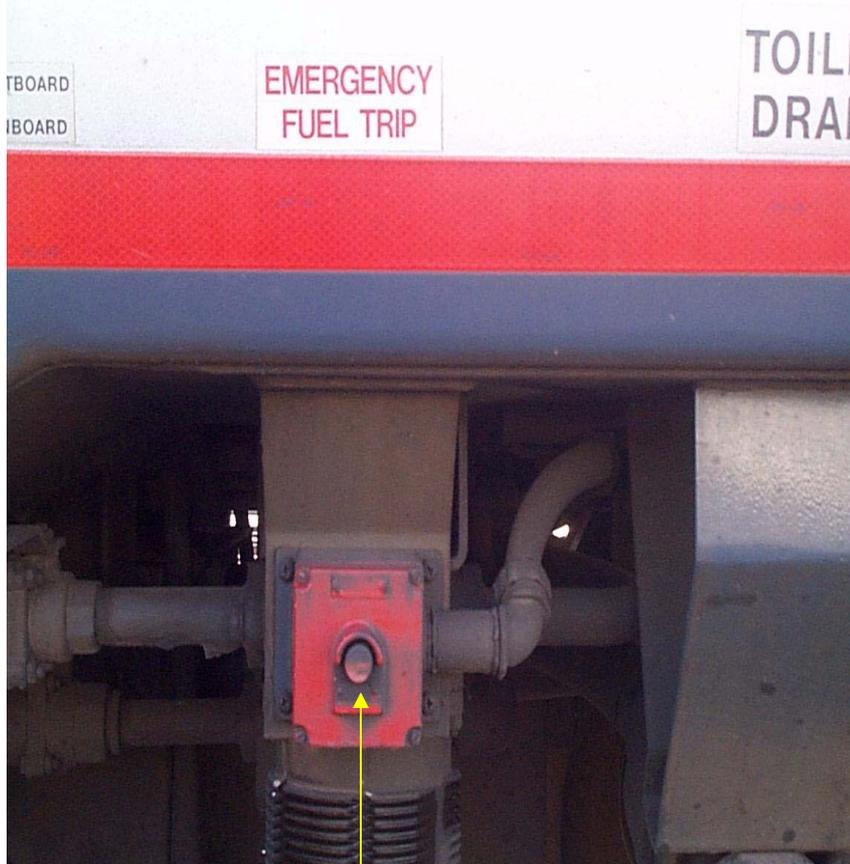
Emergency Fuel Trips (shut offs) on each side of the locomotive.
