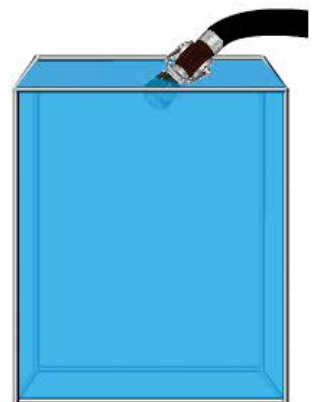
Fire Hose - 250 Gallons of Water/Minute
