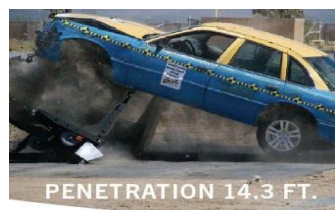
3,500lb. taxi hitting four unconnected Archer® 1200 Barriers at 30mph
