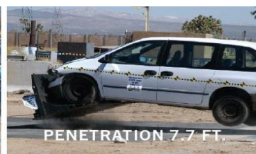
3,500lb. van hitting four connected Archer® 1200 Barriers at 30mph
